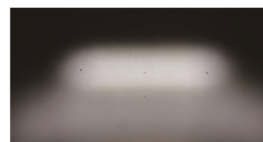
Close range light Perfect out-off line, gentle to the eyes for coming vehicles.
