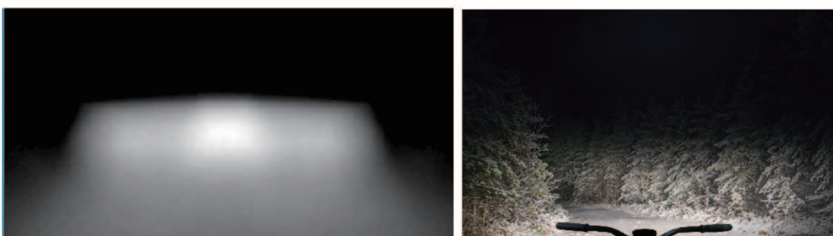
Close range light Perfect cut-off line, gentle to the eyes for coming vehicles.
